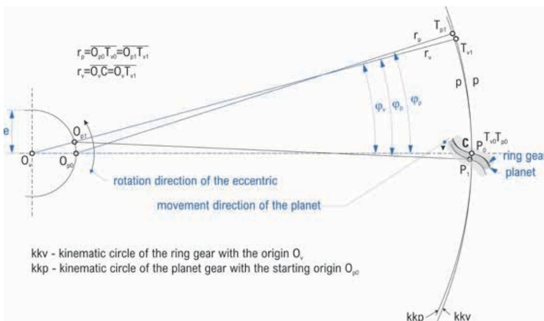
**Figure 2 :** Planetary gear movement in accordance with hypocycloid generated on the kinematic circle of the ring gear [8].
