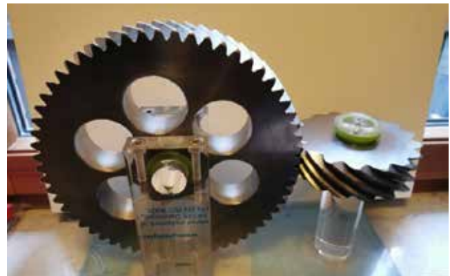
Figure 10 : A helical S-gear pair with perpendicular shafts as used in centrifuges
