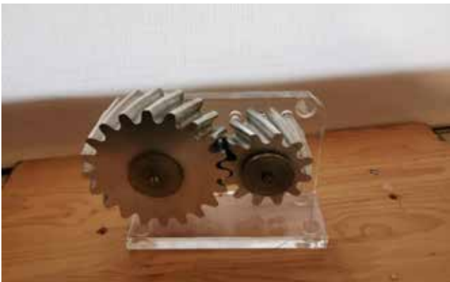
Figure 9 : A different test helical S-gear pair: driving gear z_1 = 28 , driven gear z_2 = 16
