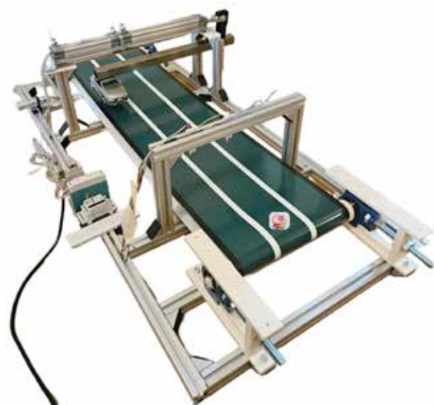
Figure 8 : Pneumatic manipulator for obstacle avoidance on conveyor belt
