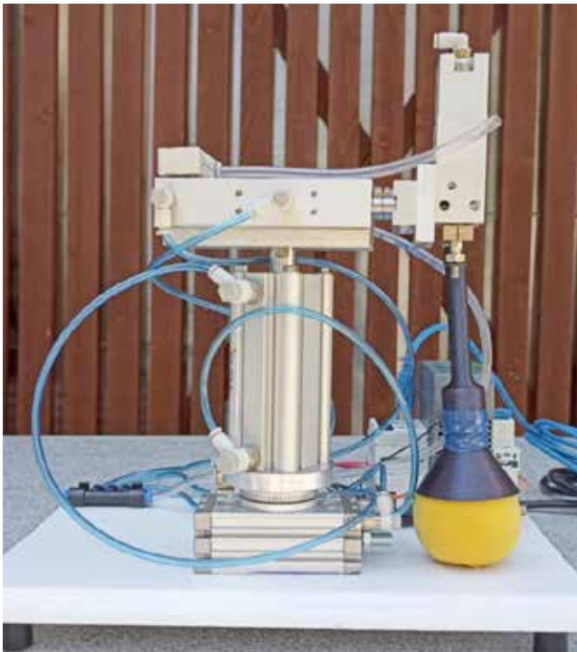
Figure 6 : Final assembly of the manipulator with the flexible gripper
