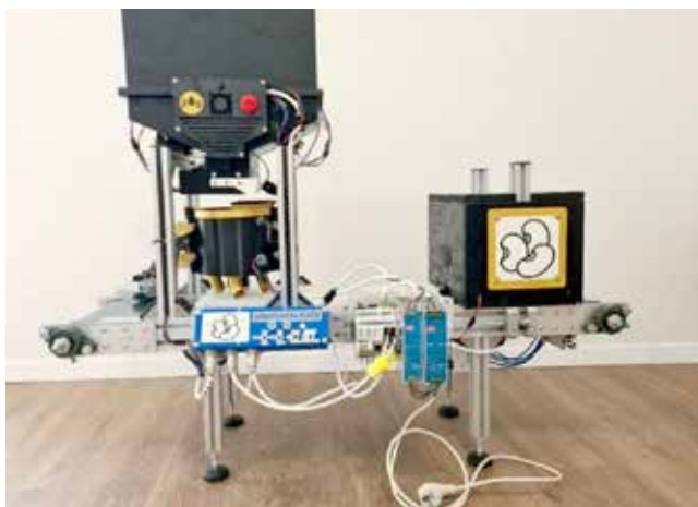
Figure 12 : Final fabricated prototype of the bean grain sorting machine
