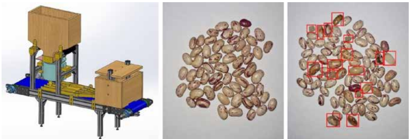
Figure 11 : CAD model of the sorting system and examples of defective bean grains
