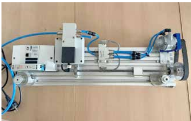
Figure 10 : Screw spindle mechanism with pneumatic drive
